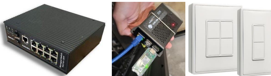
Figure 1: (a) PoE Switch; (b) COR-TAP and USB Receiver; (c) Double Rocker Kinetic Switches
