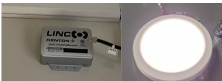
Figure 2: (a) LINC power router ; (b) DC LED Light
