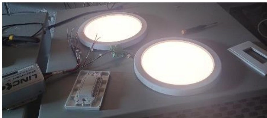
Figure 6: Multiple Lights on single output wire
